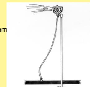
MONTAGE DIRECT SUR LA RAMPE AU SOL À L'AIDE D'UN COLLIER DE PRISE EN CHARGE OU SUR PIQUE AU SOL
